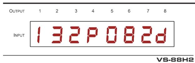
In this example: Input 1 is routed to output 1, input 3 is routed to output 2, input 2 is routed to outputs 3 and 7, a pattern is routed to output 4, output 5 is set to mute, and so on.
