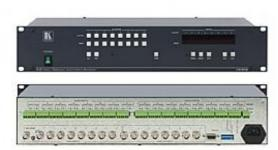
The VS-848 is a high-performance matrix switcher for composite video and balanced stereo audio signals. Switching during the vertical interval ensures glitch-free switching with genlocked sources.
