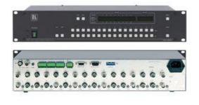
The VS-162V is a high-performance matrix switcher for composite video signals. It can also be configured as an 8x8 s-Video (Y/C) switcher, a 5x5 component (YUV) switcher, or a 4x4 RGBS switcher
