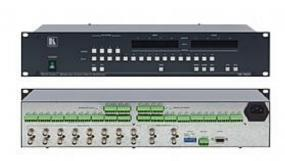
The VS-1604 is a high-performance matrix switcher for composite video and balanced stereo audio signals. Switching-during the vertical interval ensures glitch-free switching with genlocked sources.
